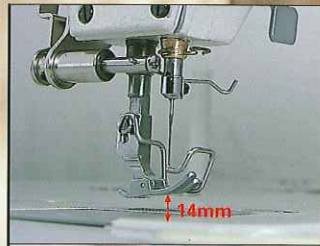
14mm lift of presser foot, highest record among the sewing machines of similar grade
